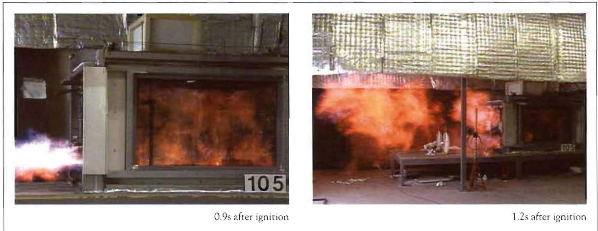
Figure 8: Backdraught from reduced ventilation opening showing a very energetic backdraught (Spark tree at rear of main compartment, switched on 6s after vents opened).
