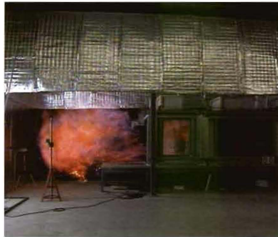
Figure 7: Backdraught with corridor section showing total flame engulfment in corridor (Spark tree at rear of main compartment, switched on 6s after doors opened. Figure shows 1.8s after ignition).
