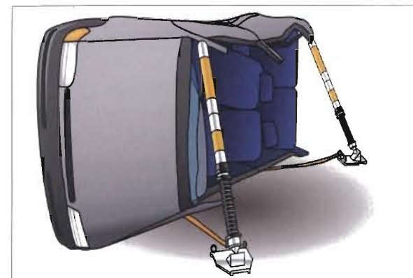
(d) Depending on the situation (i.e. limited access), it may be necessary to use shoring to stabilise the roof side of the vehicle. (Including, or instead of, the underside.)
