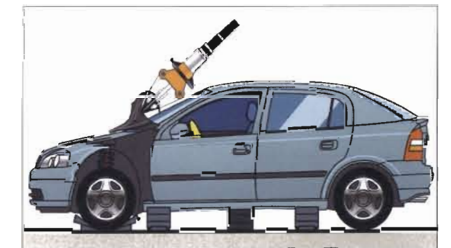
(c) Only attack one hinge at a time; do not begin between the hinges. The retaining strap will also have to be cut or spread.
