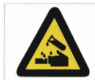
Figure 1.28 Battery electrolyte is corrosive; use appropriate personal protective equipment.
