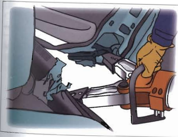
(e) Continue spreading by repositioning the spreader tips until the "B" pillar is separated from the sill or enough room has been created to complete the operation with a cutter.
