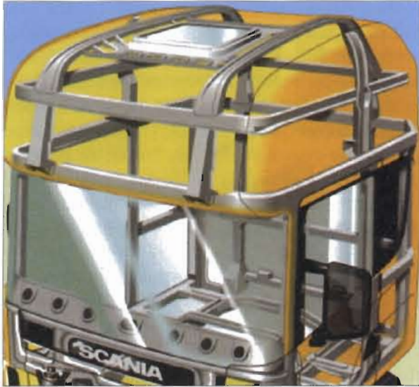
Figure 1.34 Typical Crush Resistant Cab Construction.
