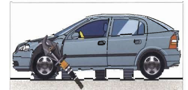
(b) Then clamp on to the wing and relocate the metal so it exposes the hinge area.
