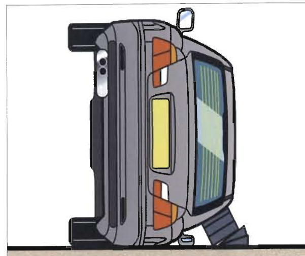
(a) Support and chock under strengthened parts of the vehicle ‘A’, ‘B’ and ‘C’ post where the gap can be seen on the ground. Think ahead; avoid placing stabilisation in areas where you are likely to cut.
