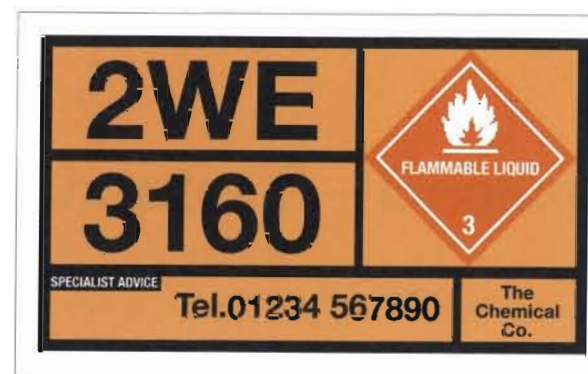
Figure 1.42 A typical hazard warning plate.
