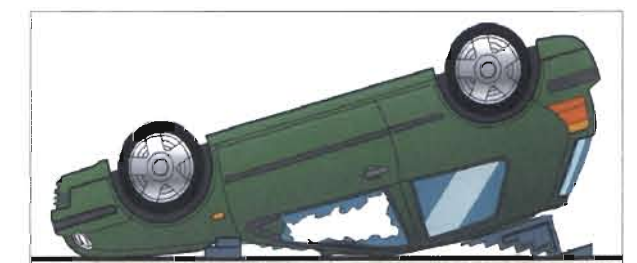
(c) Add extra blocks to the space between the engine compartment and the windscreen for added stability.
