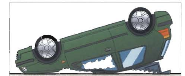
(a) Chock the space between the back of the vehicle and the ground. Note, on this occasion inverted step blocks perform their function better.
