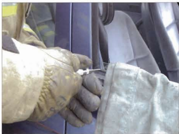
Figure 4.15 Allowing the glass to break inside the door skin.
