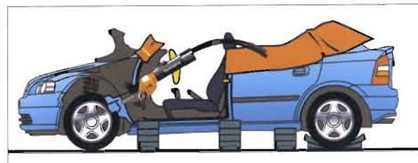
(d) Carefully introduce pedal cutter and cut away pedals as appropriate, remembering to control the loose end of the pedal to ensure it does not fly off in an uncontrolled manner.
