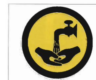
Figure 1.29 Dilute battery electrolyte spillages with copious amounts of water.
