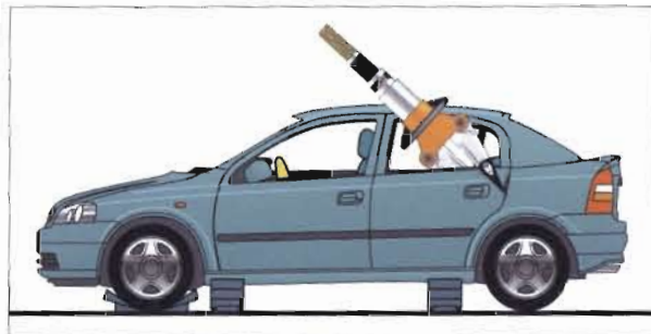
(a) Starting at the back, squeeze the door in order to create an insertion point for the tips.
