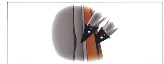
(b) If necessary, increase the opening by pinching the metal of the bottom of the door and folding downward.
