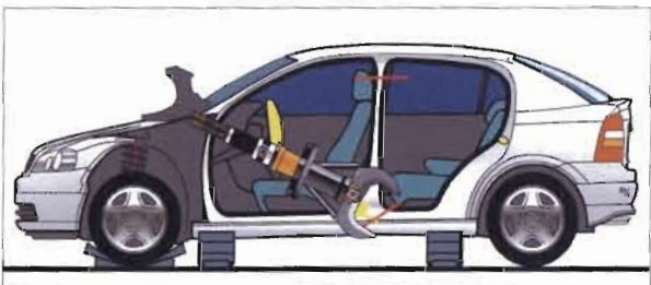
(d) Cut the top and bottom of the "B" pillar to remove it. Making the higher cut last will reduce the chance of the post moving inward and contacting the casualty.
