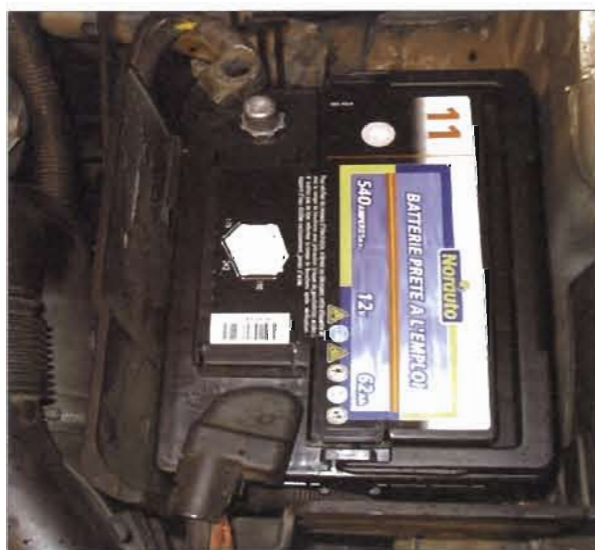
Figure 1.30 Typical battery located in engine compartment.
