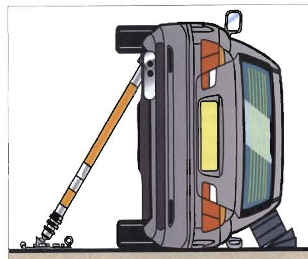
(b) Shore on the under side (the dirty side) with mechanical struts (wood, metal), or pneumatic struts. Ladders may be used to achieve comparable stability.
