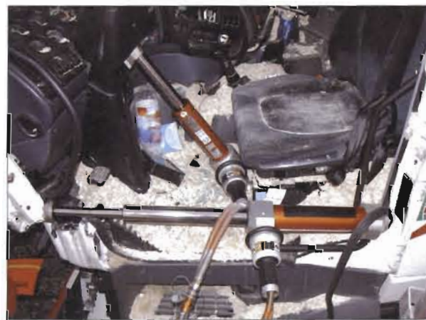
Figure 4.16 Ramming to create space.
