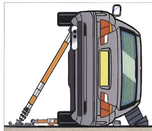
(e) When best practice is achieved, the vehicle will now have a stable base, allowing continued extrication utilising the next phase of rescue.
