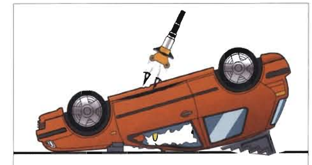
(c) Spread the door outwards away from the body, reposition the tips of the tool if the inner and outer door skin start to separate.
