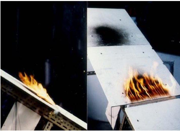
Figure 6: Diagram of the trench effect
