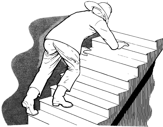
Fig. 4.1 Method of moving backwards down stairs towards a fire in a basement.
