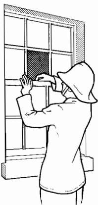
Fig. 6.15 Method of opening sash-type window when a pane has been broken. Note the left hand is holding the upper sash to prevent it falling and all jagged edges of glass have been removed from the glazing bars.
