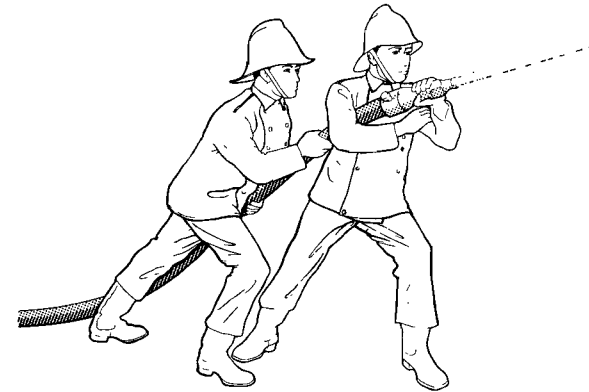
Fig. 3.7 Alternative method of holding a branch so that the weight of the charged hose is supported on the right forearm.
