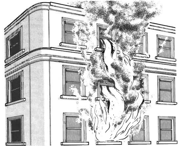
Fig 4.3 Fire can spread from floor to floor via windows which are open or which have been broken by heat.
