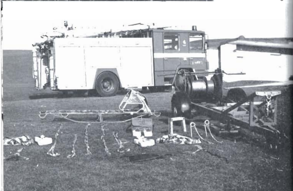
Plate 11 Cliff rescue equipment, including a winch with 150 m of 7 mm diameter cable, stretcher cable guide protector, strops and rescue slings Photo Kent Fire Brigade
