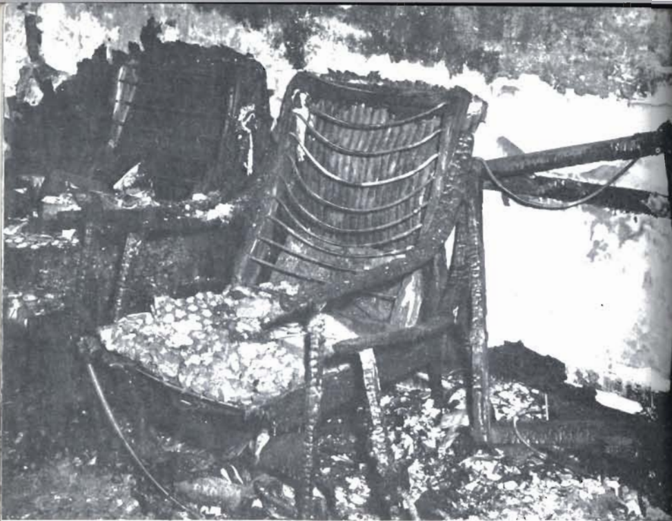
Plate 21 The different degrees to which these chairs are burnt suggests that the one on the right was the seat of the fire
