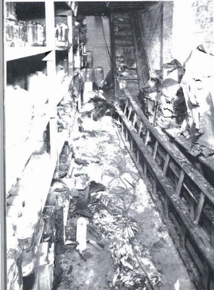
Plate 28 The removal of debris and furniture has revealed the distinctive flow pattern of an accelerant used in setting this fire. Photo: Commissioner of Police, Metropolis
