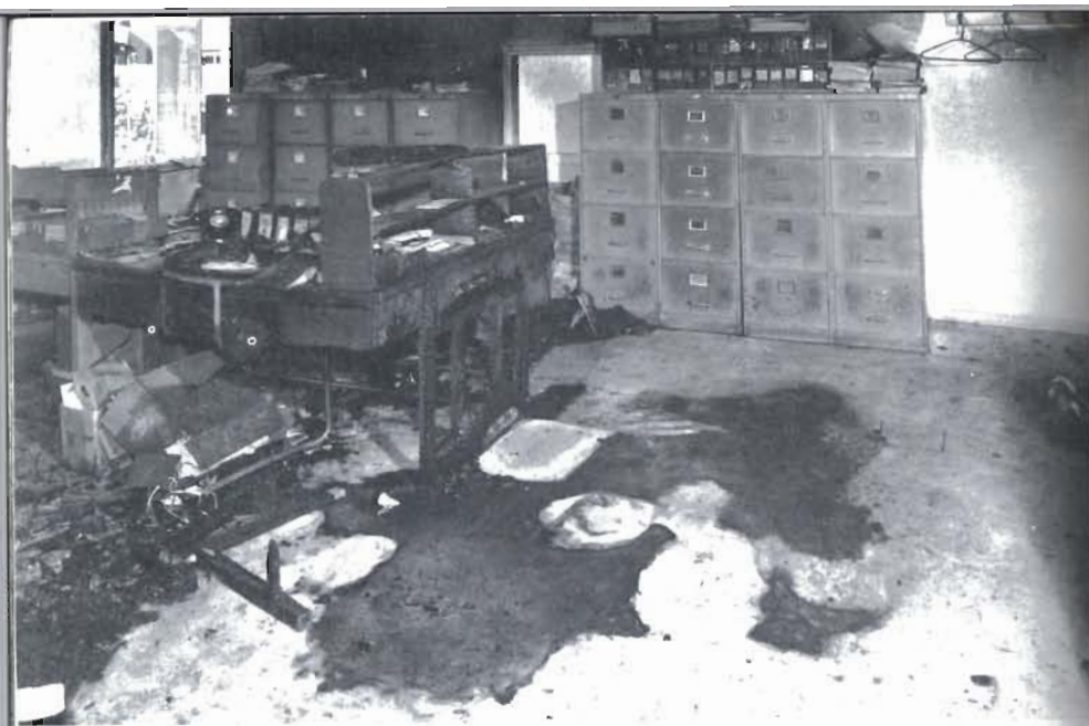
Plate 28 The removal of debris and furniture has revealed the distinctive flow pattern of an accelerant used in setting this fire. Photo: Commissioner of Police, Metropolis
