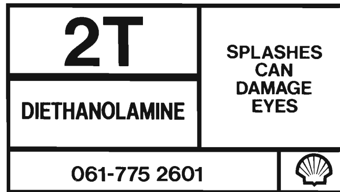
Fig. 7.11 Example of a panel giving warning of a substance of low hazard.
