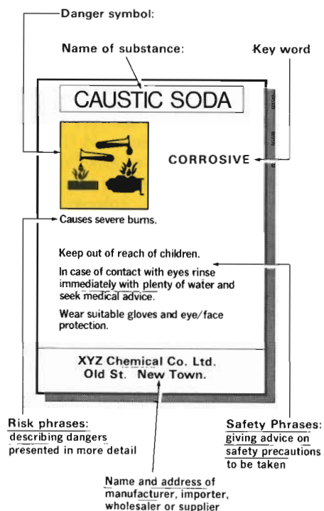
Fig. 7.7 Label for dangerous goods in a package.
