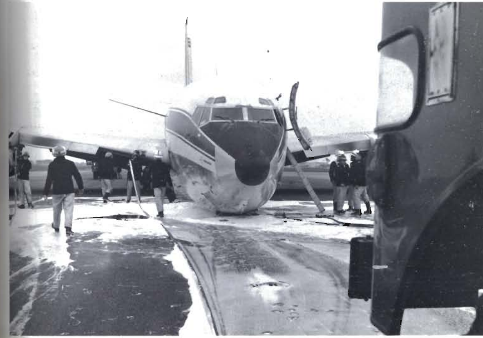
Plate A.13 Defective nose-undercarriage landing where airport fire service has laid protective foam to forestall any ignition Illustrates type of crew door which could be encountered. Photo British Airports Authority
