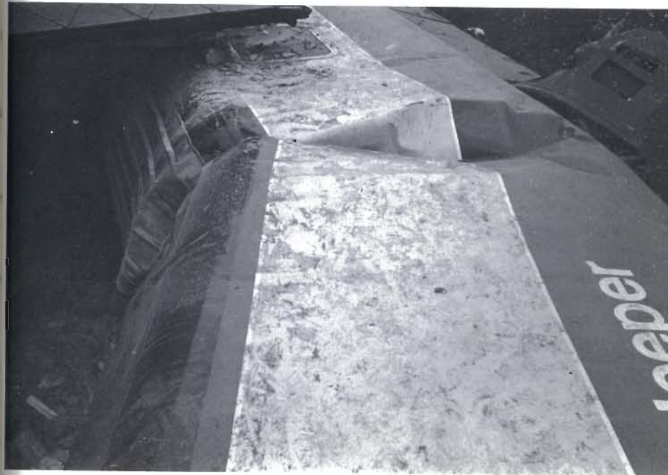
Plate R 12 This carriage struck the side of a house and crumpled. This could cause doors to jam, impeding rescue
