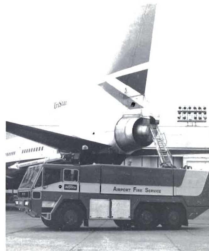
Plate A.2 Tri-Star passenger aircraft illustrating height to engine exhaust. Vehicle is a Gloster-Saro Javelin.
