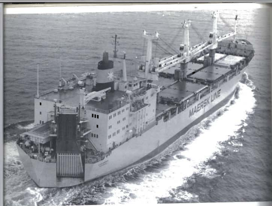
Plate S 3 21,000 tonne dwt 'Eleo Maersk' multi-purpose ship. Can be used as Ro-Ro, Sto-ro, container carrier or bulk cargo carrier Photo: Marine Publications International
