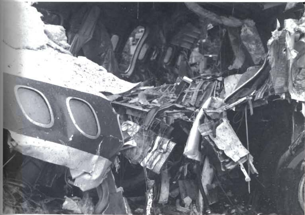
Plate A.18 An impact crash with no fire, showing examples of sheared metal
