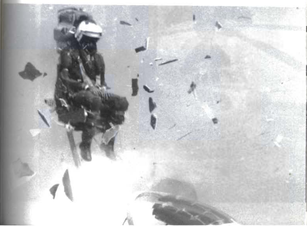
Plate A.6 Test ejection with canopy shattered by MDC about 0.7 seconds before seat fired. Front cockpit is at the initial shattering stage before ejection.
