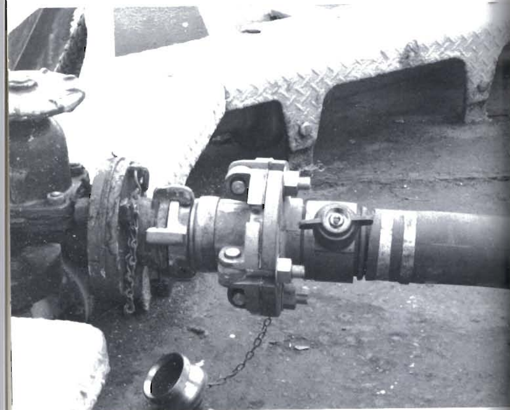
Plate S 8 An International shore connection in use. Photo: Hants Fire Brigade
