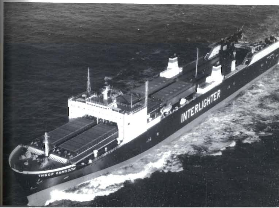
Plate S.2 Modern LASH ship, 35,800 gross tonne, USSR 'Tibor Szamuely' Photo: Skyfotos Ltd.
