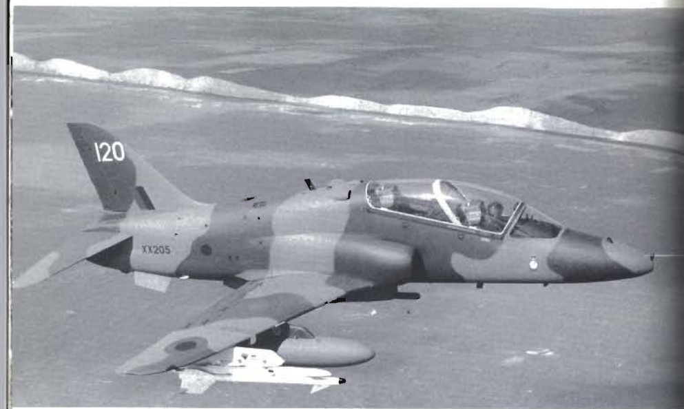
Plate A 20 Hawk 2-seat attack aircraft with Sidewinder missile and cannon. Compare with Plate A 23 Photo British Aerospace
