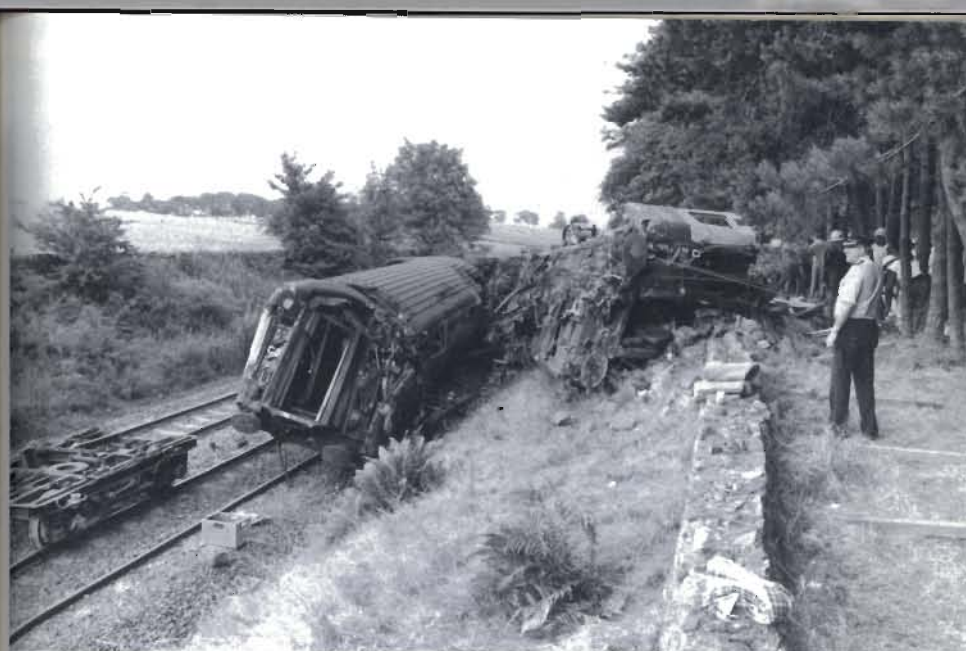
Plate R 7 Passenger coach on embankment secured by Tirfor equipment during rescue operations Photo: Daily Record, Glasgow
