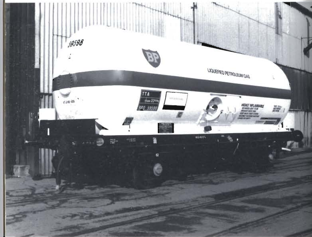
Plate R 14 A typical LPG tank wagon with a white barrel and horizontal orange stripe Photo Standard Railway Wagon Co
