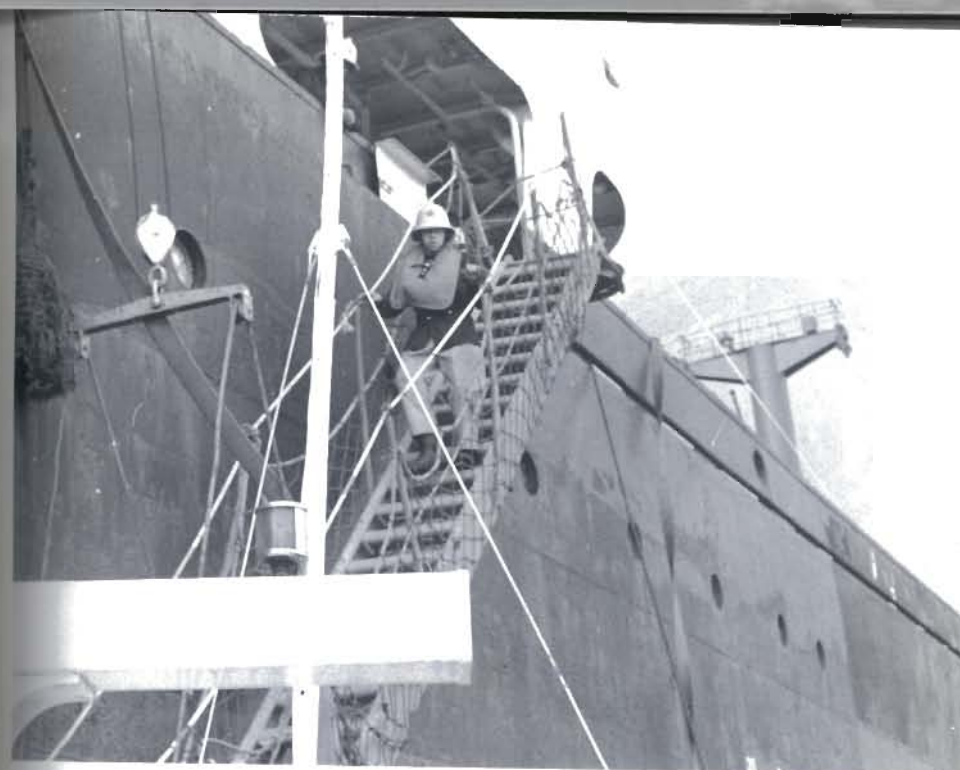
Plate S.26 Illustrating the height, steepness and narrowness of access to this ship's main deck in this case all gear had to be either hauled aboard or manhandled up this companionway Photo Essex Fire Brigade
