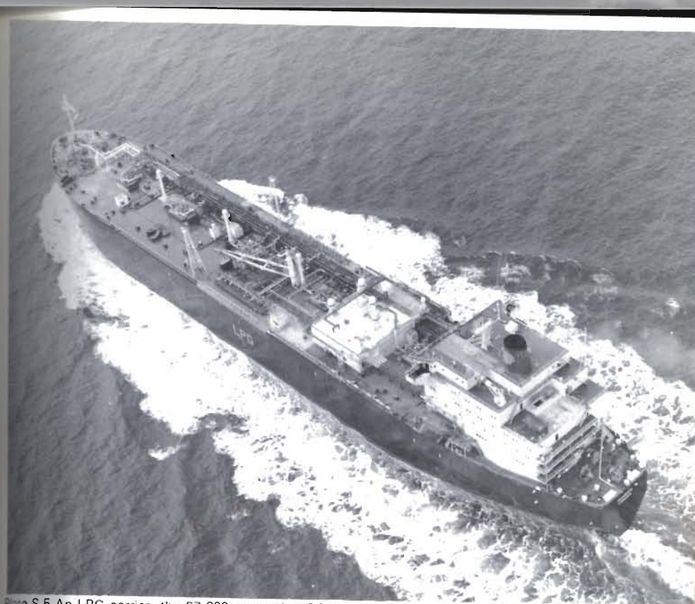
Plate S.5 An LPG carrier, the 37,000 tonne dwt SS 'Isomeria', gas capacity 58,950 m 3 , fitted with self-supporting pressurised and refrigerated tanks Photo: Harland and Wolff Ltd
