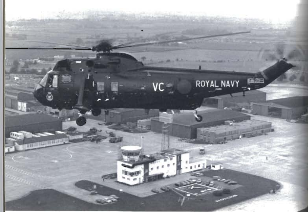
Plate A.11 Mk 4 Sea King helicopter of the Royal Navy Various delineated panels and doors can be seen. Photo Royal Navy
