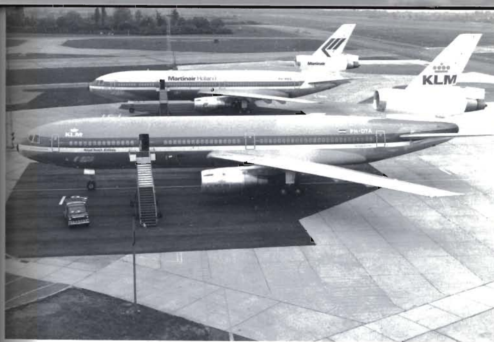
Plate A.1 Two DC-10 aircraft showing fore and aft passenger loading doors, overwing exits and crew exits
