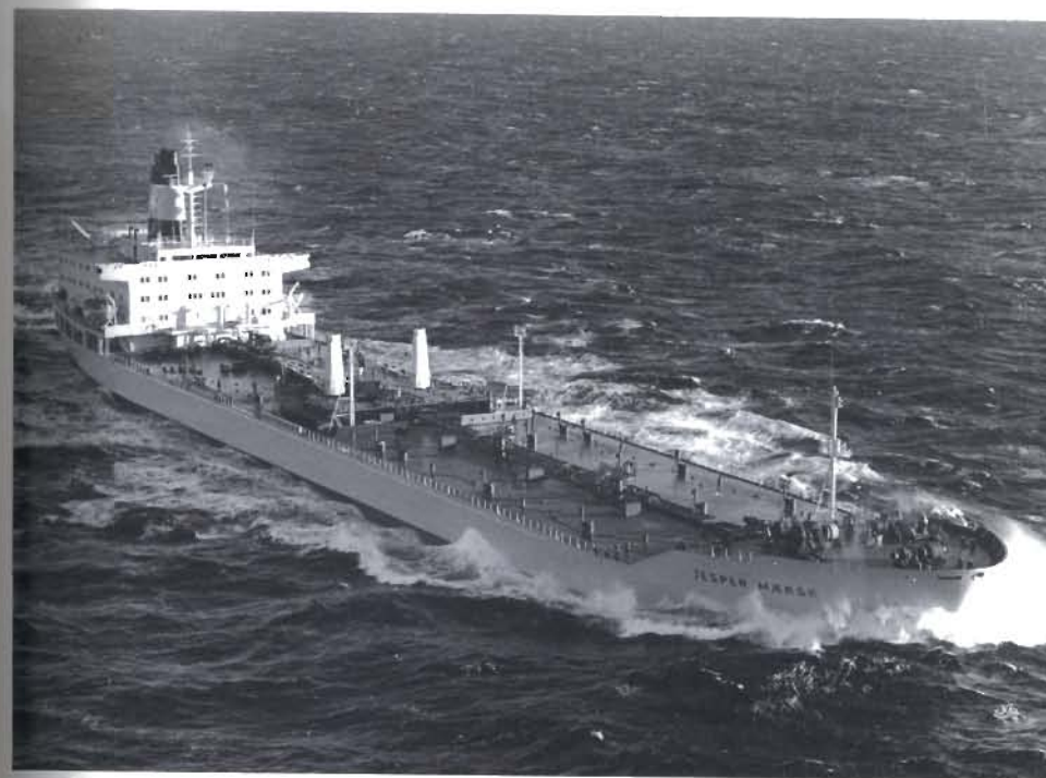
Plate S.18 A gas carrier with a capacity of 12,000 m 3 Note the firefighting platforms at intervals along the centre of the deck Photo. Marine Publications International
