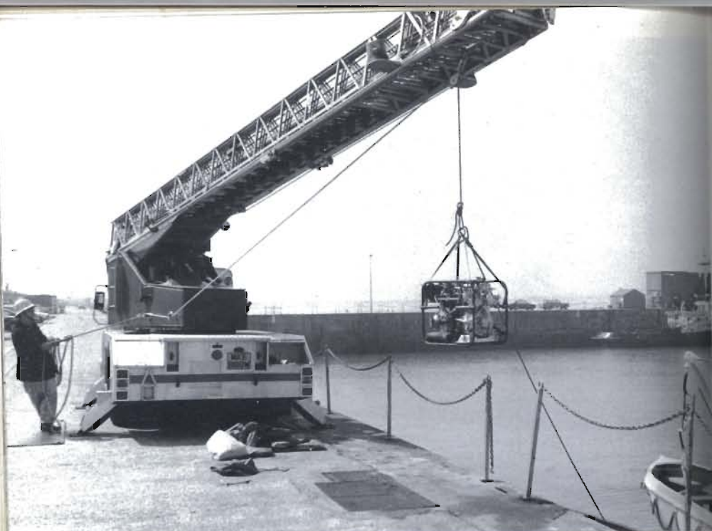
Plate S.20 A turntable ladder being used as a crane to load gear onto a tug Photo Kent Fire Brigade
