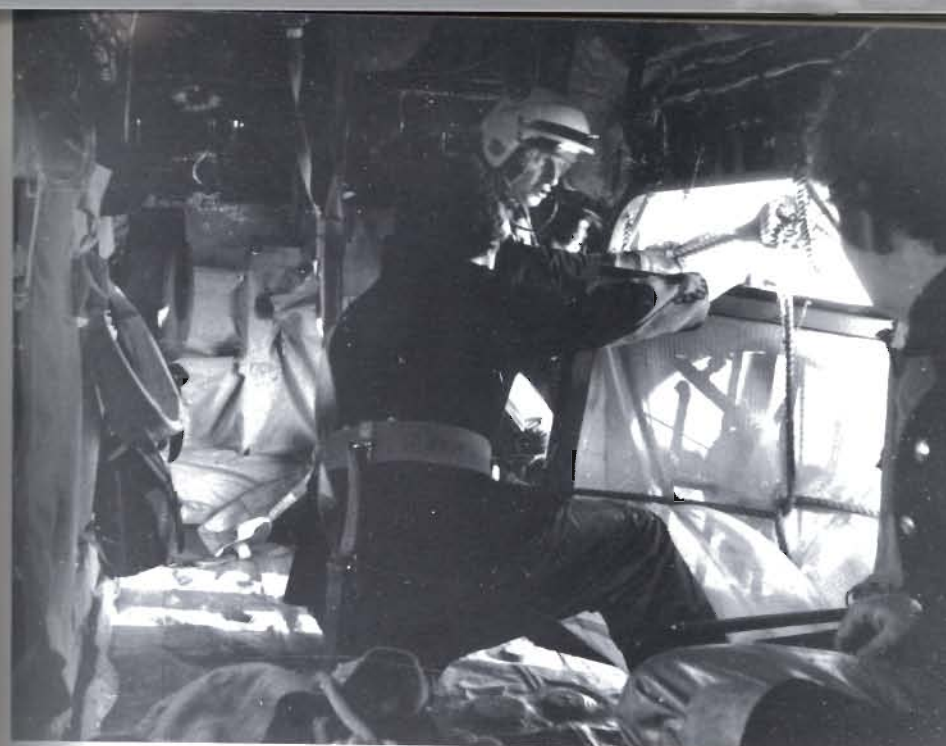
Plate S.22 Firemen and RAF aircrew preparing to lower a high expansion foam unit onto a ship's deck. The very restricted space is obvious as is the safety harness Photo C P Nelson
