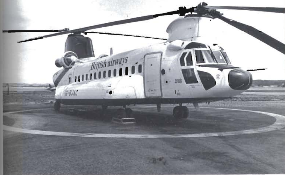
Plate A.9 Boeing Vertol 234 Note the droop of the forward rotor, the rear escape hatch and the cutaway delineation. The bulges at the bottom of the fuselage contain fuel tanks. Also see Plate A.10. Photo: British Airports Authority
