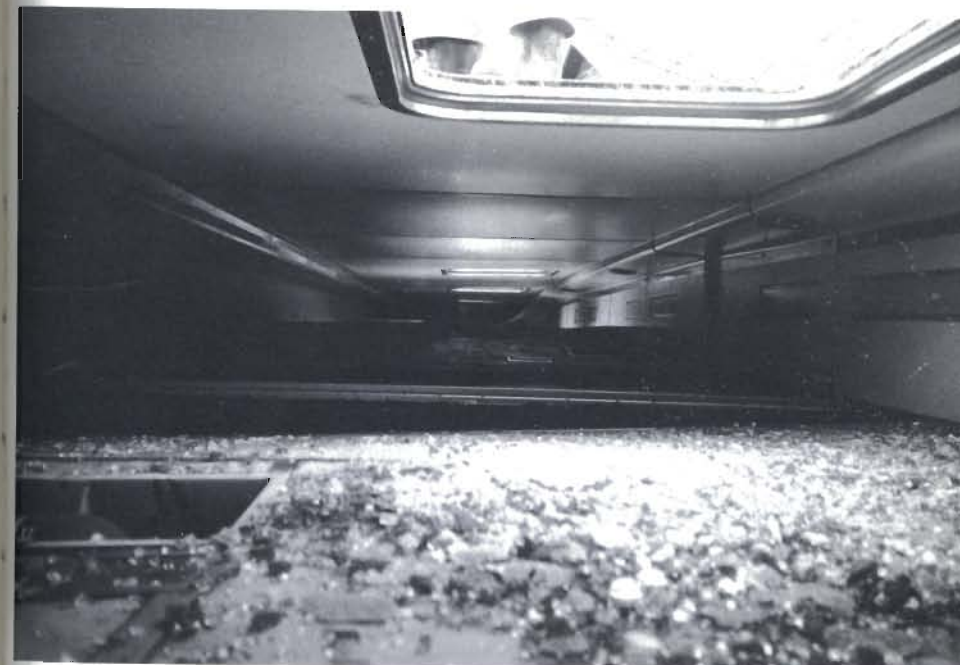
Plate R 11 View along the corridor of an overturned sleeping car showing the restricted access to the compartments. The roof is to the right
