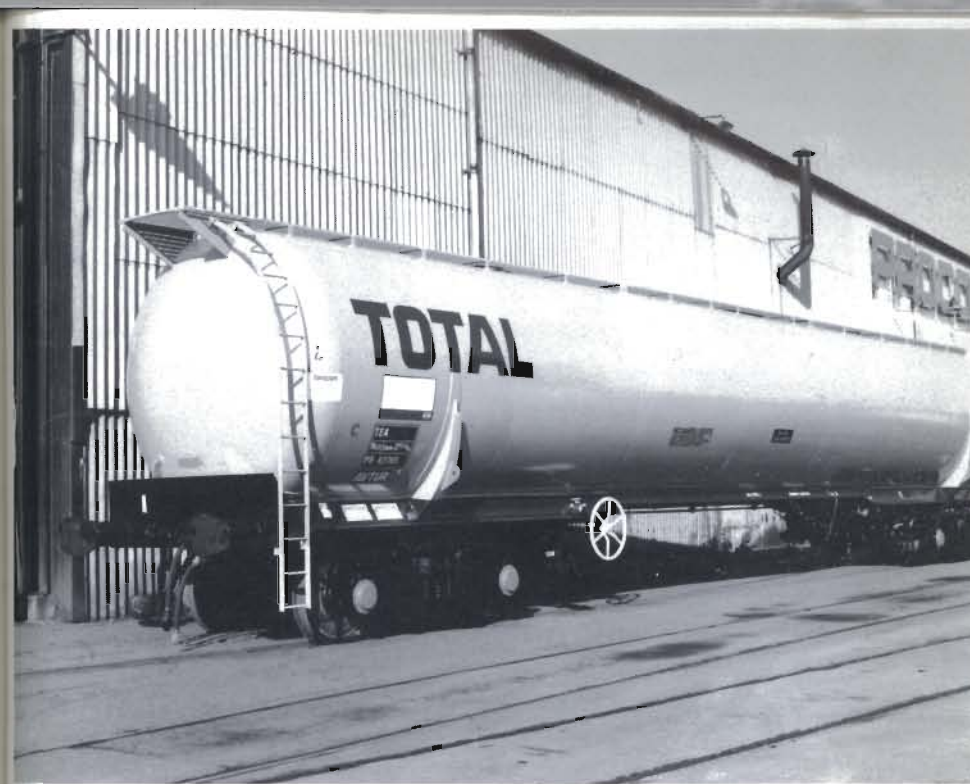
Plate R 15 Tank wagon used to carry AVTUR aviation fuel Photo Standard Railway Wagon Co
