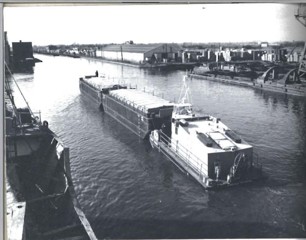
Plate S.24 A push-tow formation Depending on the size of the waterway either a maximum of 3 barges or 6 barges can make up the load Photo British Waterways Board
