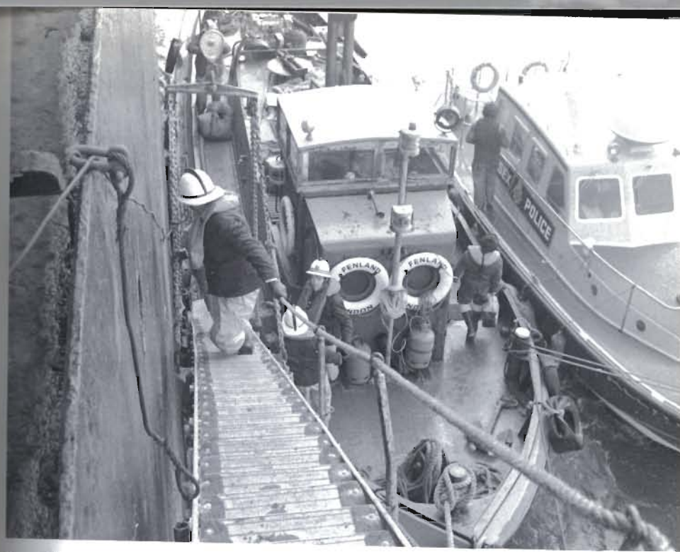
Plate S.13 At this incident the small tug 'Fenland' was used for the initial boarding and remained as a pumping platform. The police vessel acted as the ferry for equipment, reliefs etc. Note the narrow companionway. Photo: Essex Fire Brigade
