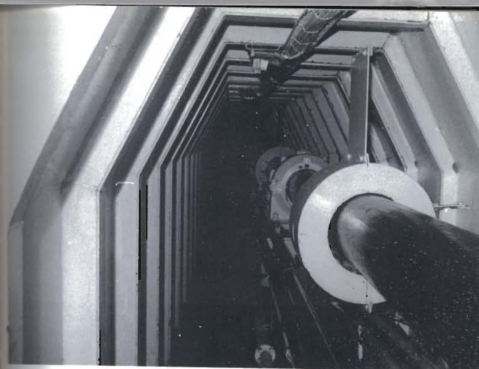
Plate S.1 A typical shaft tunnel leading to an engine room amidships. Photo: Essex Fire Brigade
