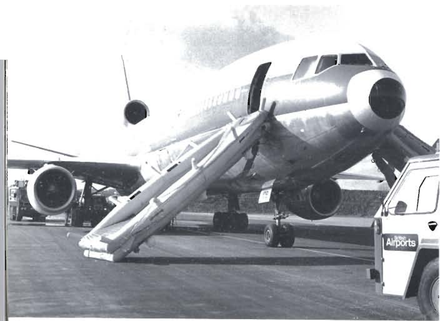
Plate A. 15 Good example of DC-10 deployment of an escape chute. The sheer height of the aircraft doors from ground level is worth noting. Photo: British Airports Authority
