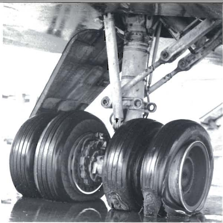
Plate A. 14 Typical tyre failure on multi-wheel undercarriage. The massive suspension can be clearly seen. Photo: British Airports Authority
