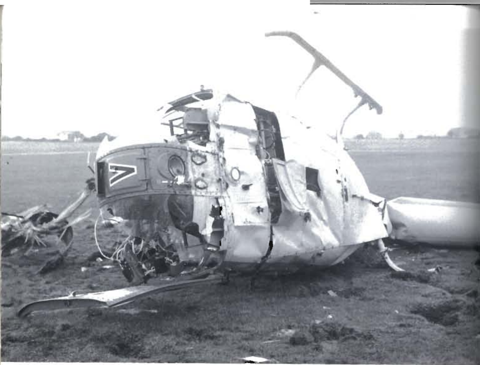
Plate A 24 Heavy landing of a helicopter. The lightness of construction can be easily seen. Photo Royal Air Force
