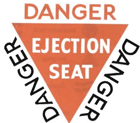
Fig. 2.4 Sign on side of fuselage denoting ejection seat.
