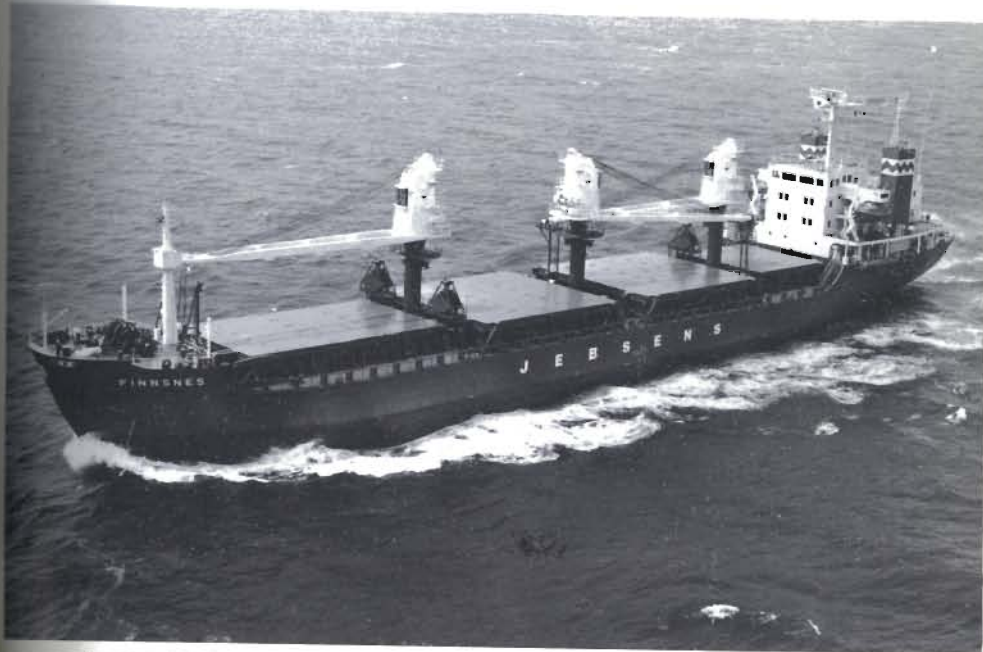
Plate S.6 A general bulk carrier of 8,000 gross tonne Photo: Marine Publications International
