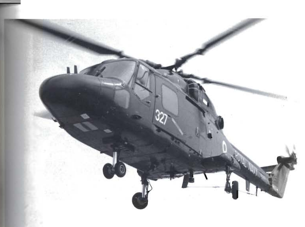
Plate A.12 Royal Navy Lynx helicopter The means of access is clearly marked The tail rotor of this aircraft would be very low Photo Royal Navy
