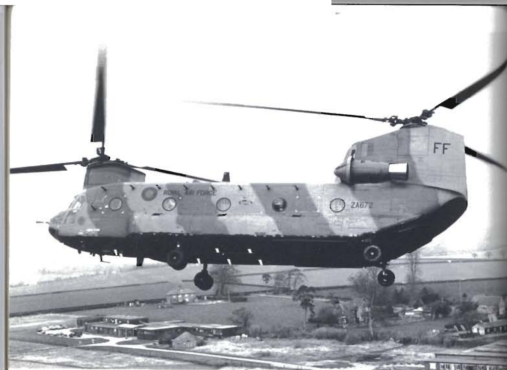
Plate A.10 The Chinook which can be compared with its civil version in Plate A 9 Note the break-in panel and escape hatch Photo Ministry of Defence
