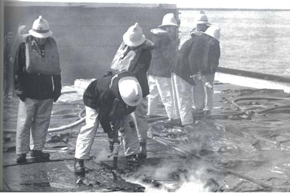
Plate S.27 A fire in a tightly packed cargo of building board When the cargo was eventually unstowed the cause was found to be a fixed lighting installation which had been left permanently switched on Photo Kent Fire Brigade
