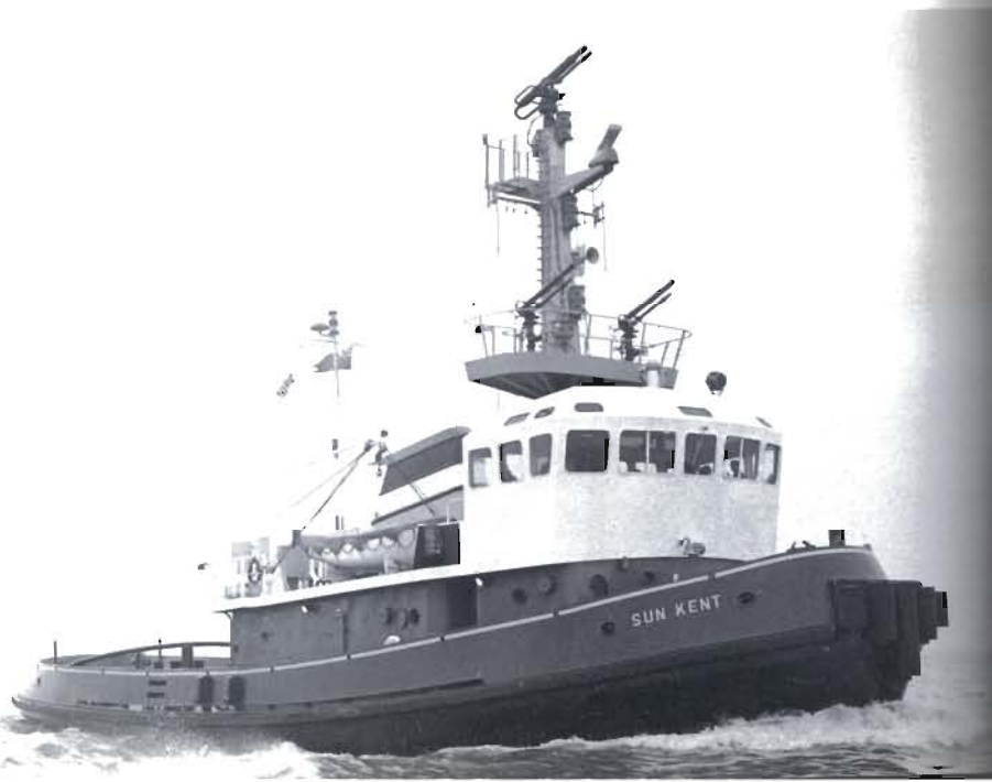
Plate S 12 A fire tug equipped with three monitors capable of a water or foam attack. Photo: Alexandra Towing Co Ltd
