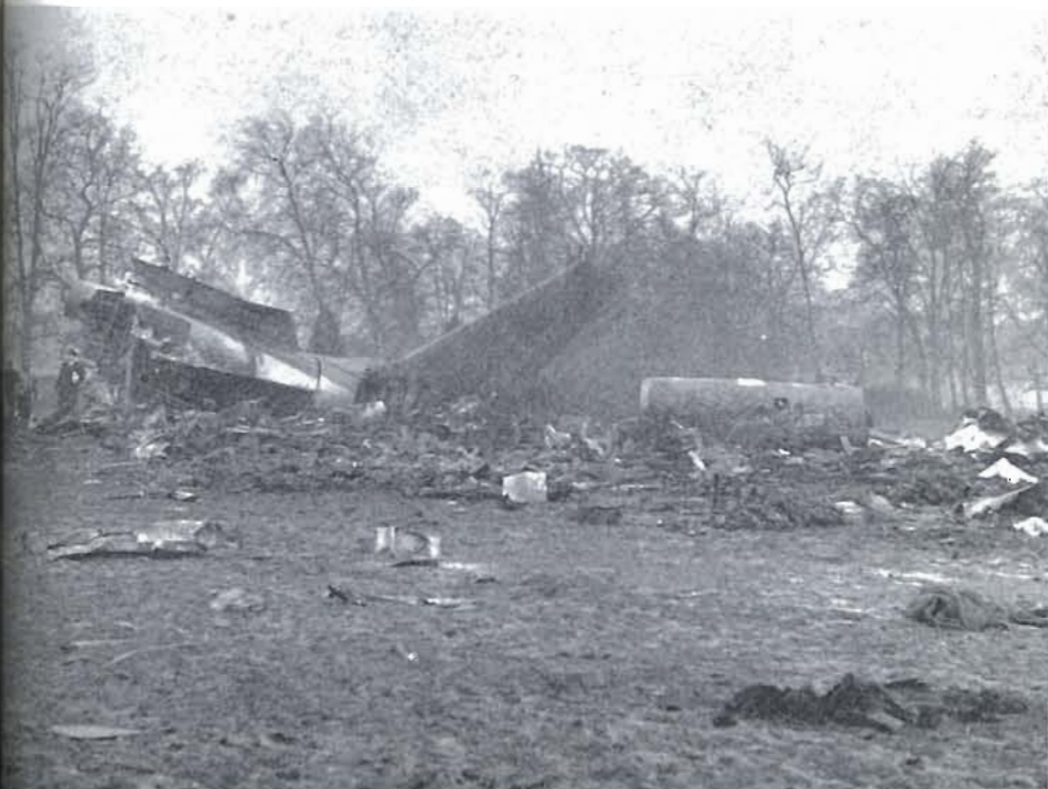
Plate 77. A Boeing 727 which crashed at Gatwick Airport in January 1969. Forty-five people were killed, but 12 survived. The picture shows how wreckage can be strewn over a large area.
