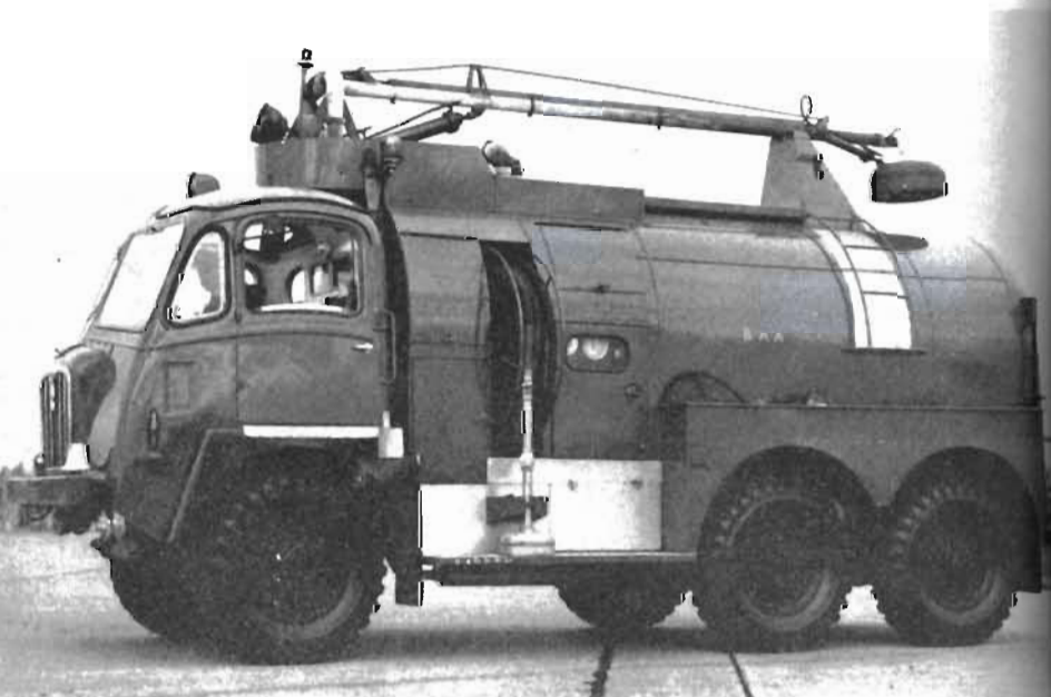
Plate 71. The Cardox appliance of BAA which can discharge \text{CO}_2 from the specially-designed boom applicator whilst the vehicle is in motion.
