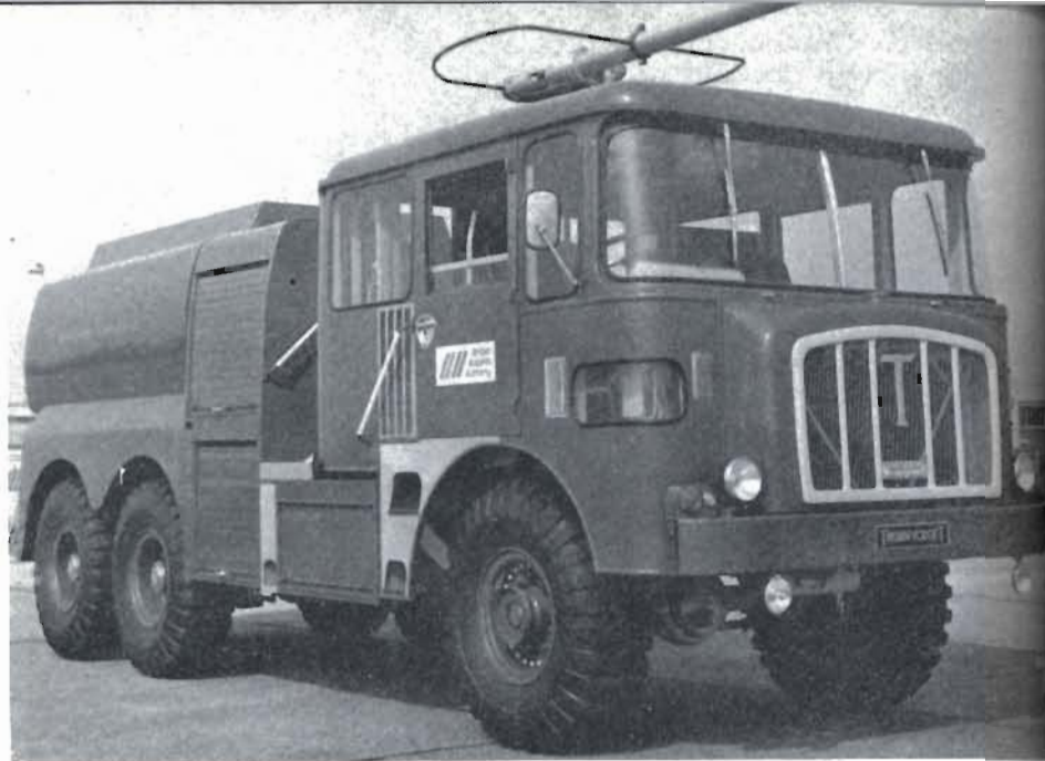
Plate 70. One of British Airport Authority's fire-fighting appliances, the Nubian Major, with the foam monitor mounted on the roof.
