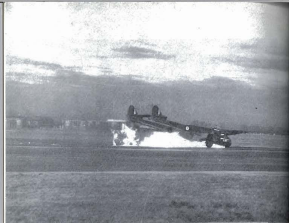
Plate 80. A military aircraft landing on its nose, as a result of which fuel tanks have ruptured and burst into flames.
