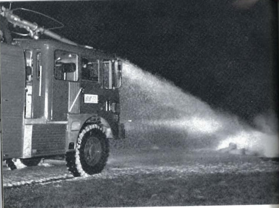
Plate 74. The Nubian Major appliance producing foam. The monitor is controlled and directed by a member of the crew from the position behind the cab.
