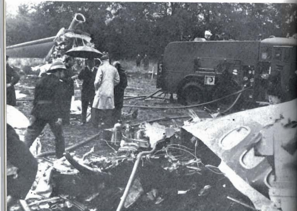
Plate 84. In this Trident crash the aircraft broke in two with the fuselage and tailplane finishing 100 yards (91.4 metres) apart.
