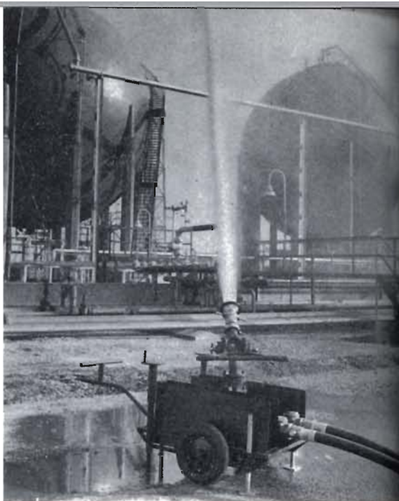
Plate 103. A light portable trailer-mounted water monitor being demonstrated. This can deliver a stream of water or a wide curtain of diffused water at 500 gallons (2,273 litres) a minute.
