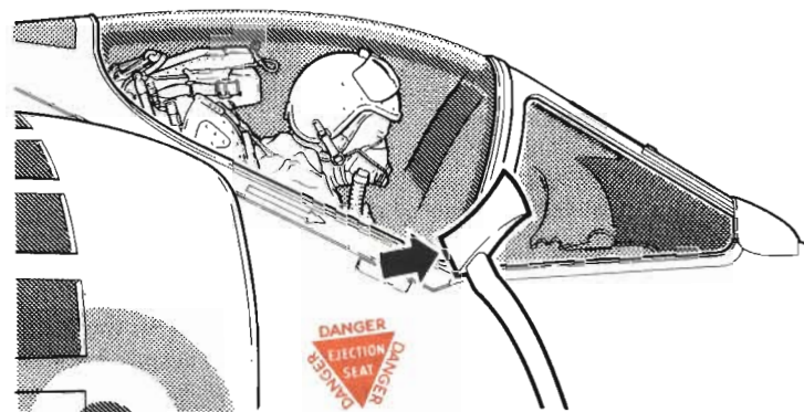
Fig. 4-21. Method of breaking in through the perspex canopy using a large axe.
