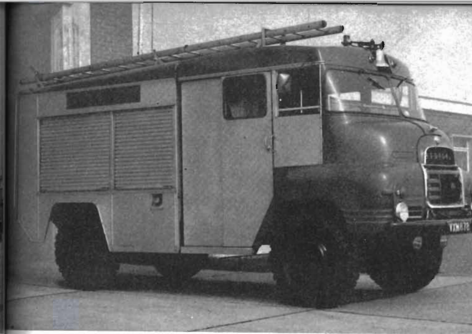
Plate 72. A typical civil airport rescue tender. This appliance carries the necessary equipment for effecting a quick rescue at aircraft accidents.
