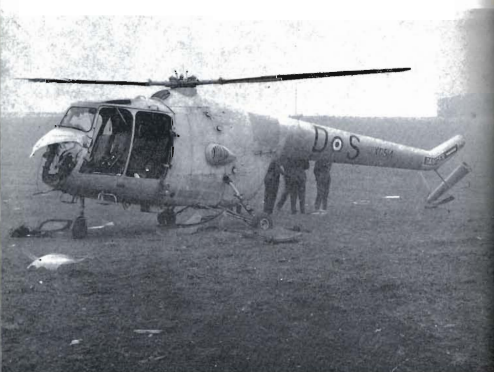
Plate 88. Because of its light construction a helicopter is easily damaged when a crash occurs.
