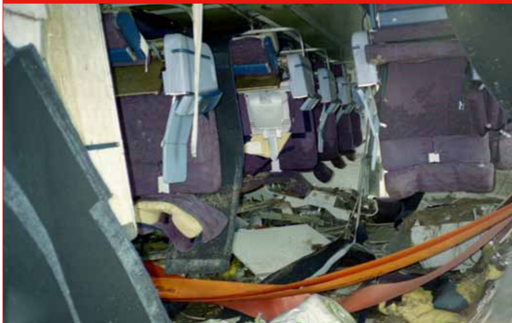
Picture 1: Internal hazards following an inverted aircraft accident
