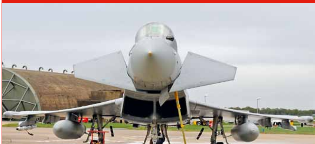
Picture 9: Typhoon under fuselage engine intakes
