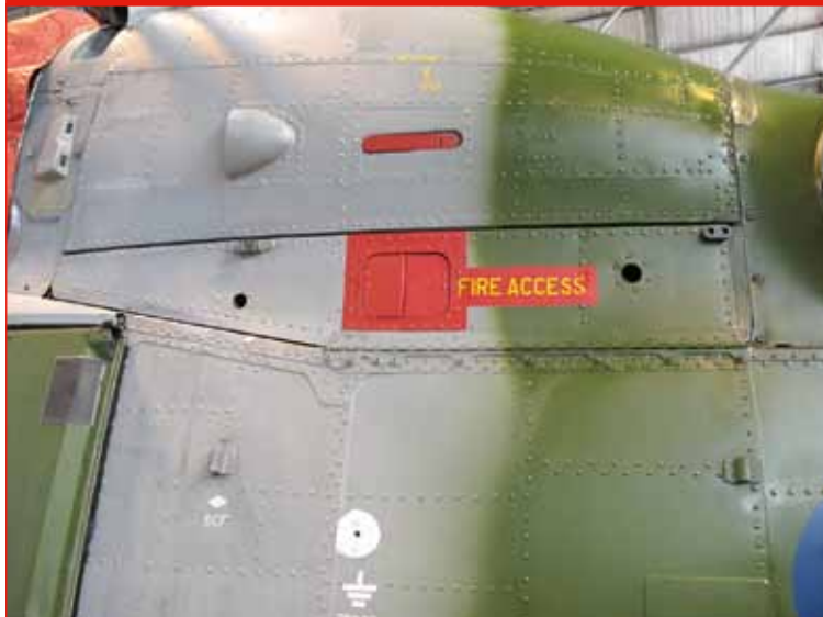
Picture 8: Flap fire access panel on a Lynx helicopter
