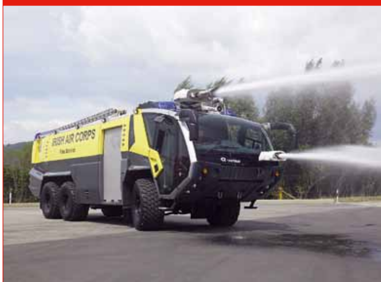
Picture 3: Panther Rescue and Fire Fighting Service vehicle demonstrating roof and bumper monitors
