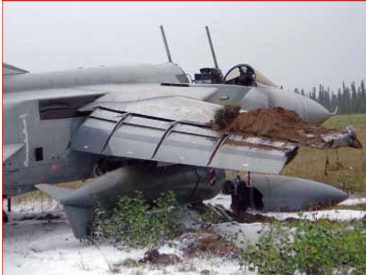
Picture 37: Crashed Tornado, both pilots ejected and the guide rails from the cockpit are clearly visible
