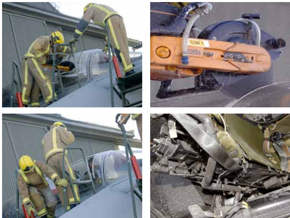
Picture 30, 31, 32 and 33: Forced entry being made into a cockpit by DFRMO firefighters, final pictures indicates the amount of dust produced as a result of this activity
