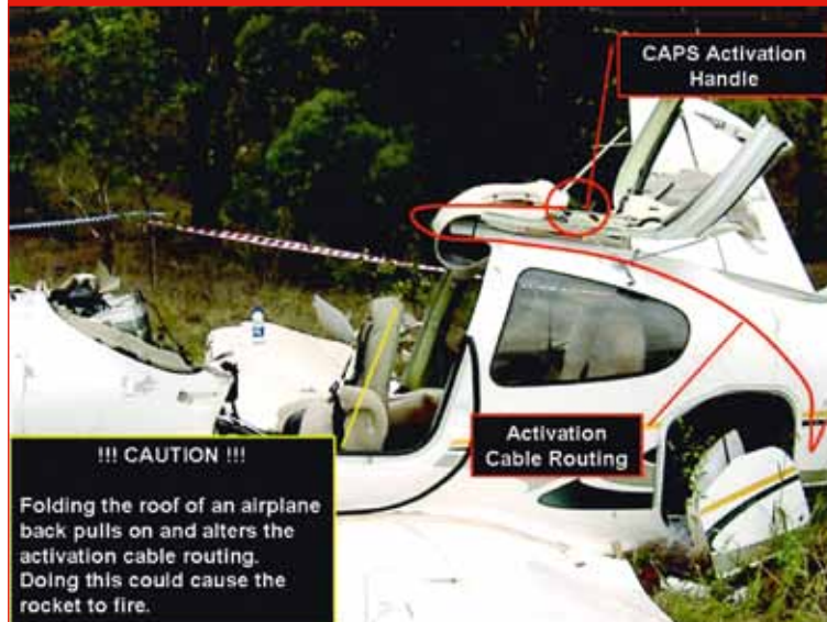
Picture 20: Demonstrates the potential hazards associated with cutting an airframe fitted with a ballistic parachute system
