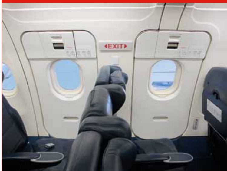
Picture 11: Example of over wing exit hatches on a narrow bodied aircraft
