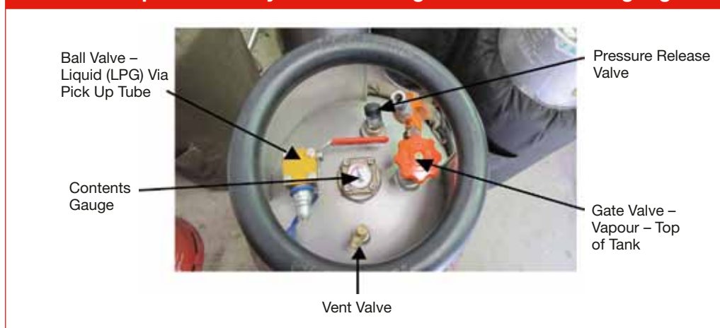
Picture 5: Top view of a cylinder showing control valves and gauges
