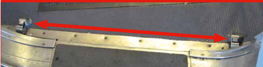
Picture 8: Girt bar securing clips located on the floor inside the aircraft door
