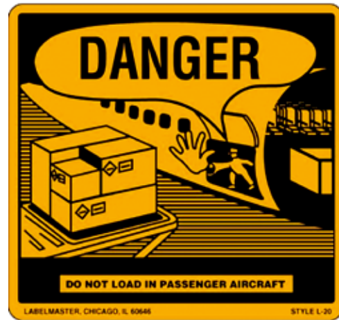
Picture 7: Identification label for cargo that cannot be loaded on passenger aircraft
