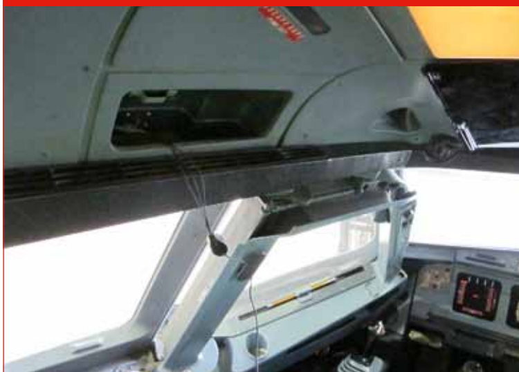
Picture 12: Flight deck pilot escape window with escape rope located in compartment above
