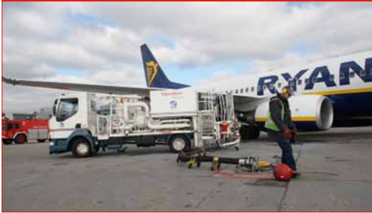
Picture 22: Refuelling vehicle at Gatwick using the fuel hydrant system
