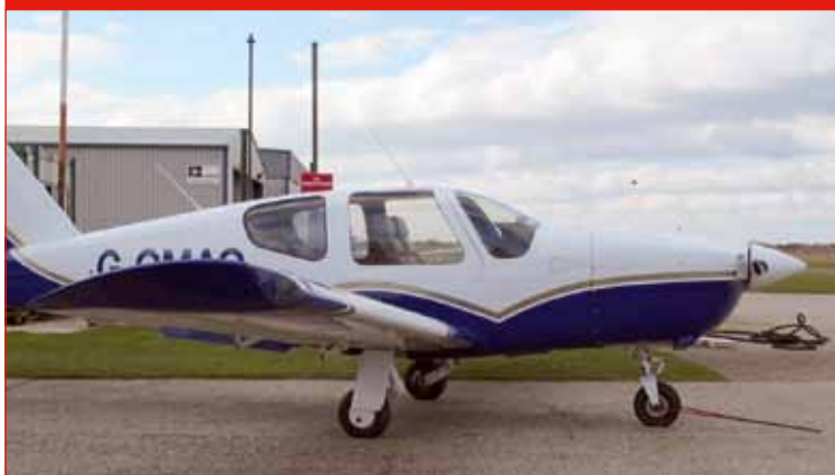
Picture 4: Low wing configuration
