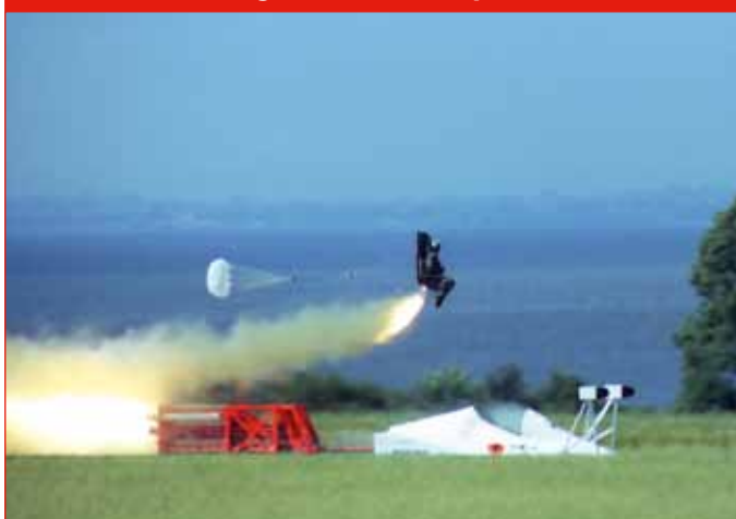
Picture 36: Drogue chute in operation
