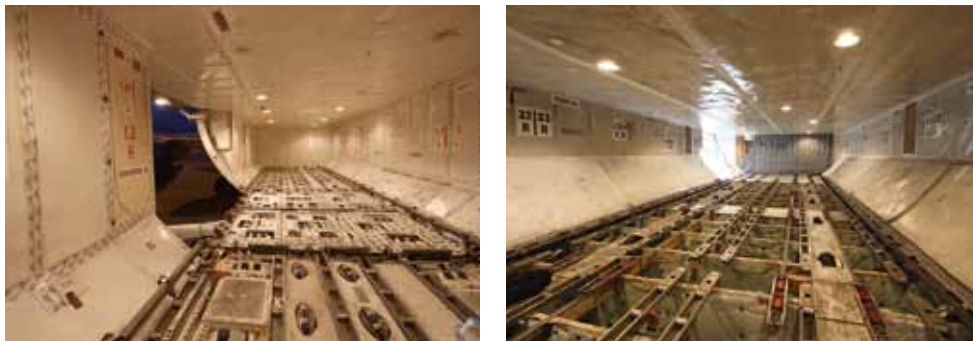
Pictures 5 and 6: Internal floor layouts/hazards of aircraft holds
