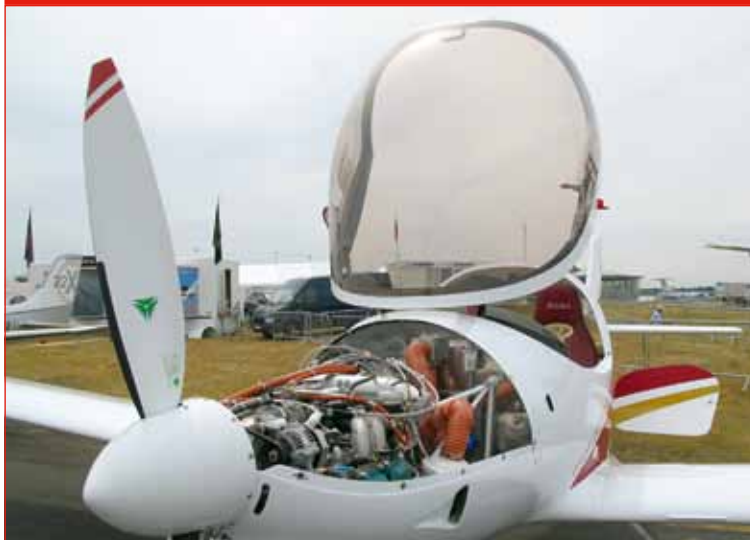
Picture 1: Typical piston engine on a light aircraft with a fire resisting bulkhead separating the engine compartment from the cockpit
