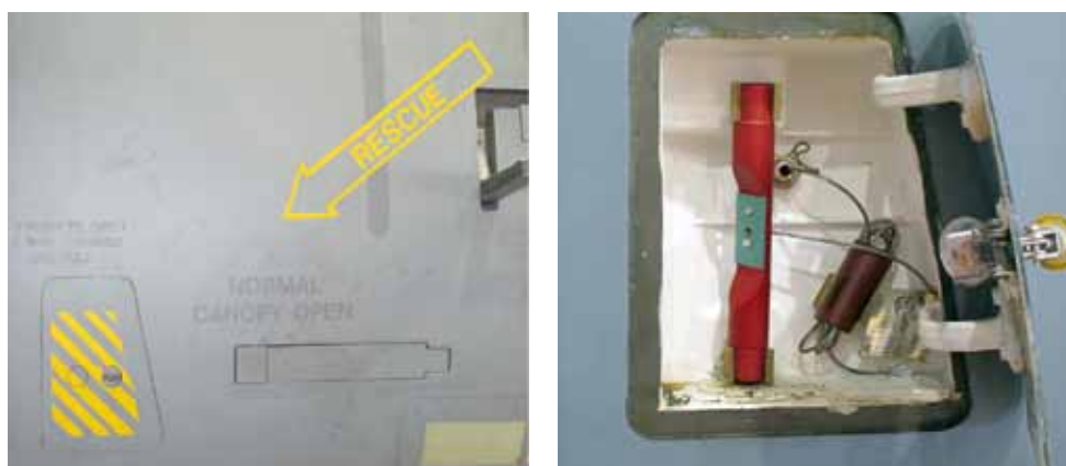
Picture 27, 28 and 29: Emergency instruction and emergency canopy release cable on a Harrier
