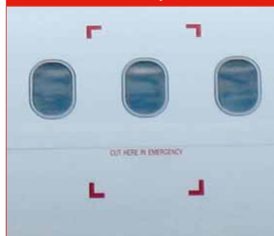
Picture 14: Break in point
