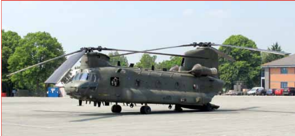
Picture 18: Demonstrates rotor blade height from the ground for a Chinook helicopter
