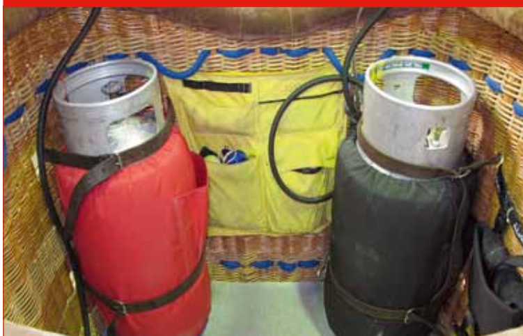
Picture 4: Two propane cylinders strapped into basket
