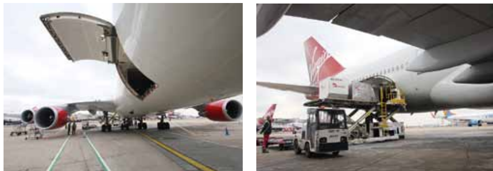
Pictures 3 and 4: Example of typical cargo bay door (top hinged)
