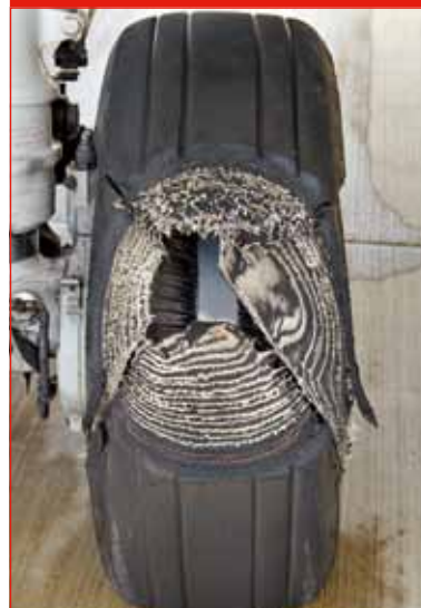
Picture 2: Burst tyre as a result of heavy braking
