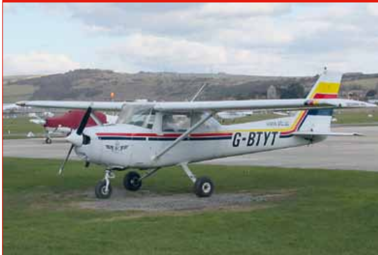
Picture 3: High wing configuration
