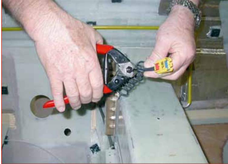
Picture 34: Third method to cut the cable connecting the electrical module assembly to the inflator assembly
