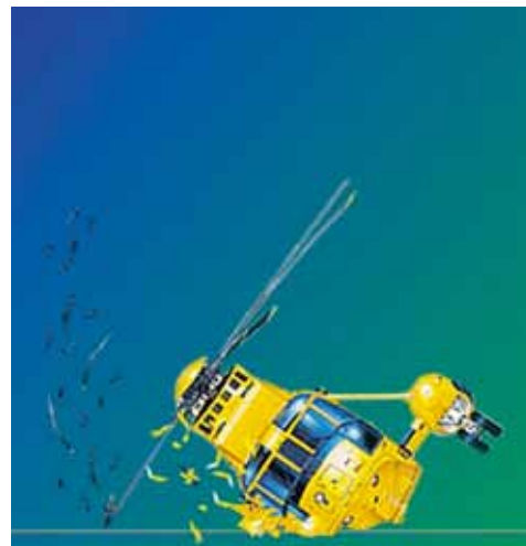
2. Full structural failing of undercarriage assembly, rotor blades shatter as they make contact with the ground.
