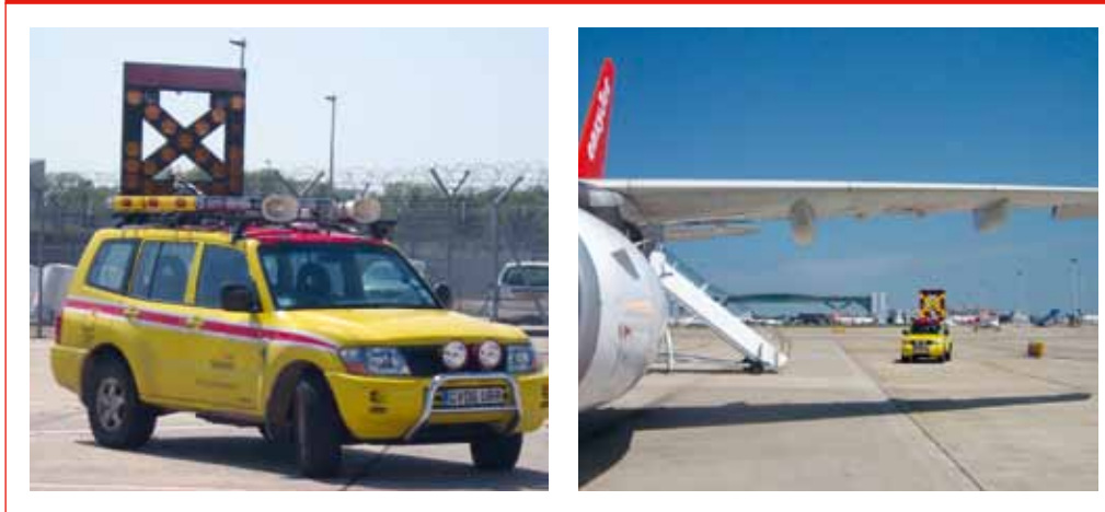
Pictures 3 and 4: Passenger evacuation management system, carried on an airport ground operation vehicle
