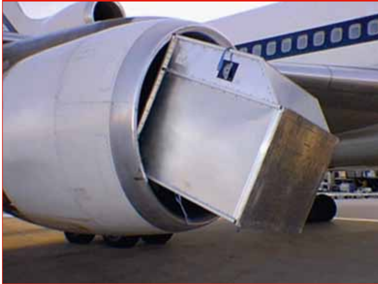
Picture 15: Cargo container drawn into engine demonstrating the power of engine suction
