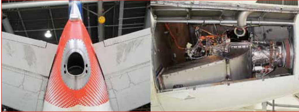
Pictures 18 and 19: Auxiliary power unit exhaust port and auxiliary power unit viewed through an open inspection panel
