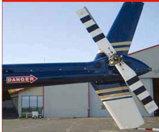
Picture 10: Traditional tail rotor
