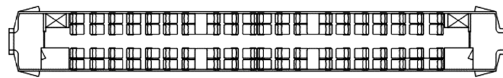
Plan – luggage stack and toilet each end, internal sliding door between vestibule and saloon
