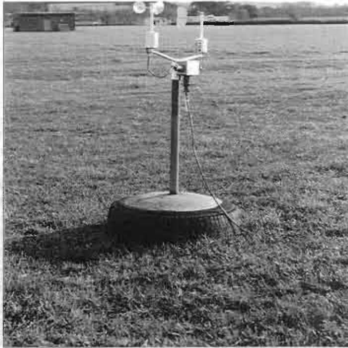
Figure 10 : Wind sensors mounted at 1m
