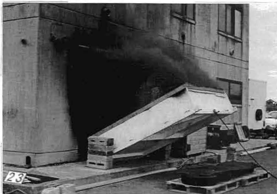
Figure 12 A Smoke Retaining Box being removed from a French Window Opening during a Trial
