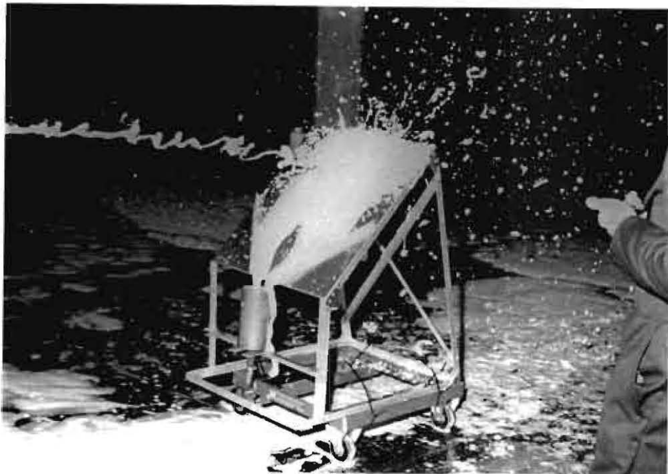
Figure 12 : Branch Trolley Showing Deflector in the Up Position
