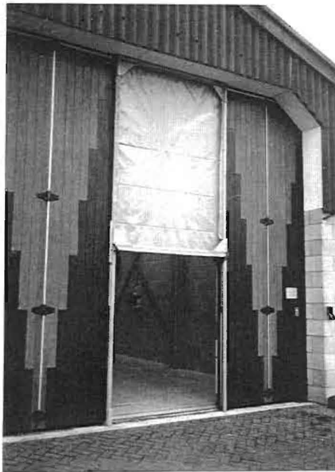
Figure 18. Doorway defining blank in position in F E U garage.
