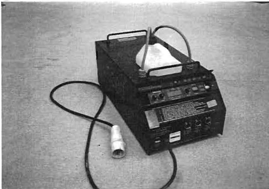
Figure 6. LeMaitre 'G-300' cold smoke generator.
