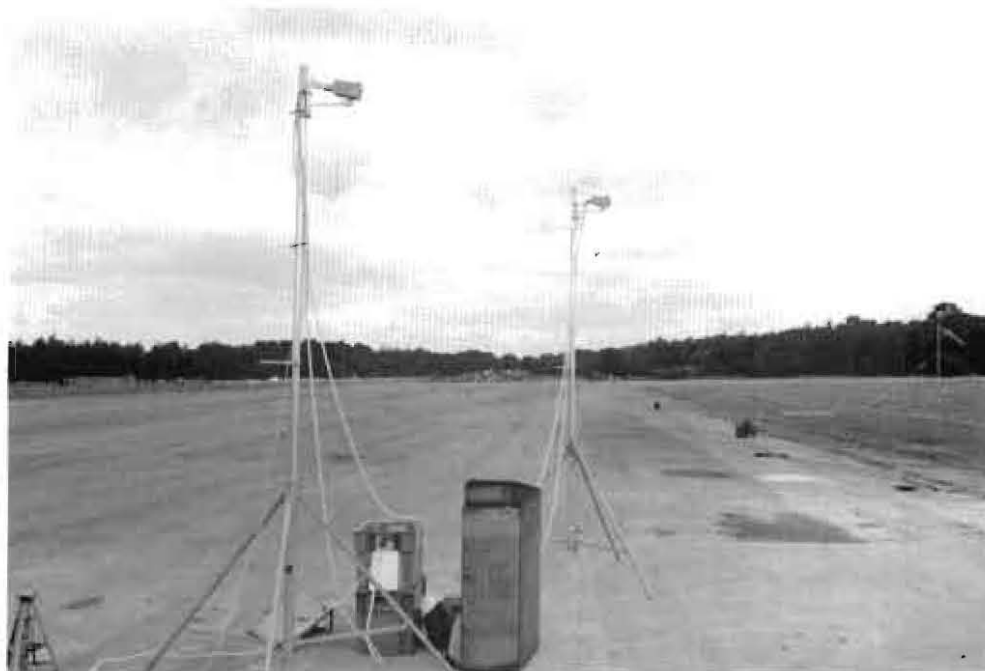
Figure 10: Two radiometers mounted on masts
