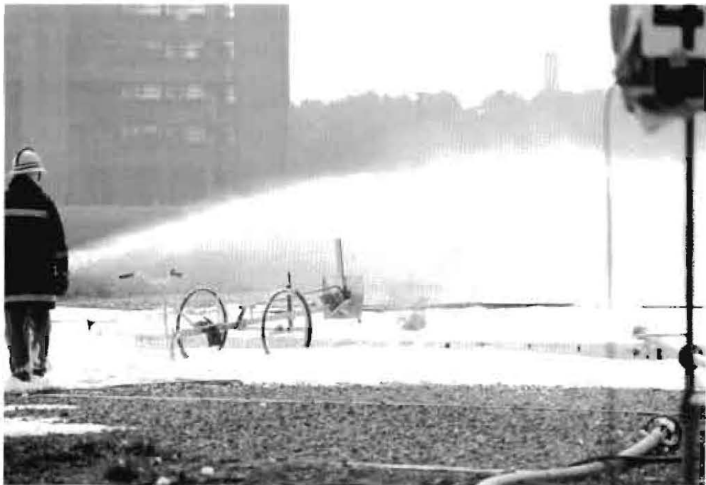
Figure 17: Burnback rig in position for burnback test
