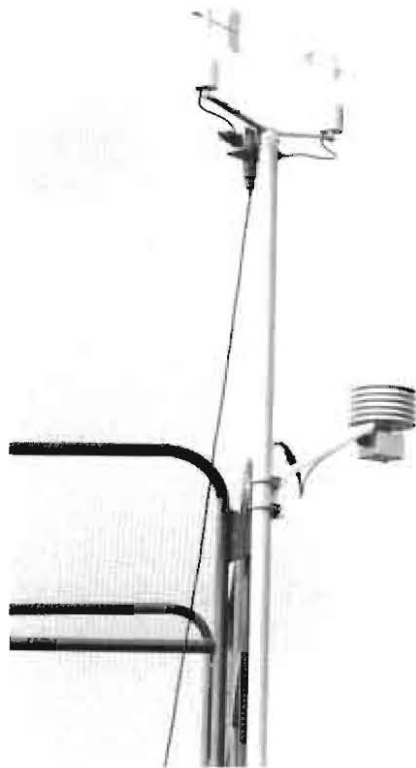
Figure 6: Wind speed, wind direction, air temperature and humidity sensors
