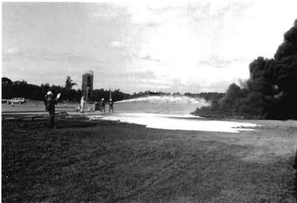
Figure 15: Foam stream being applied to fire
