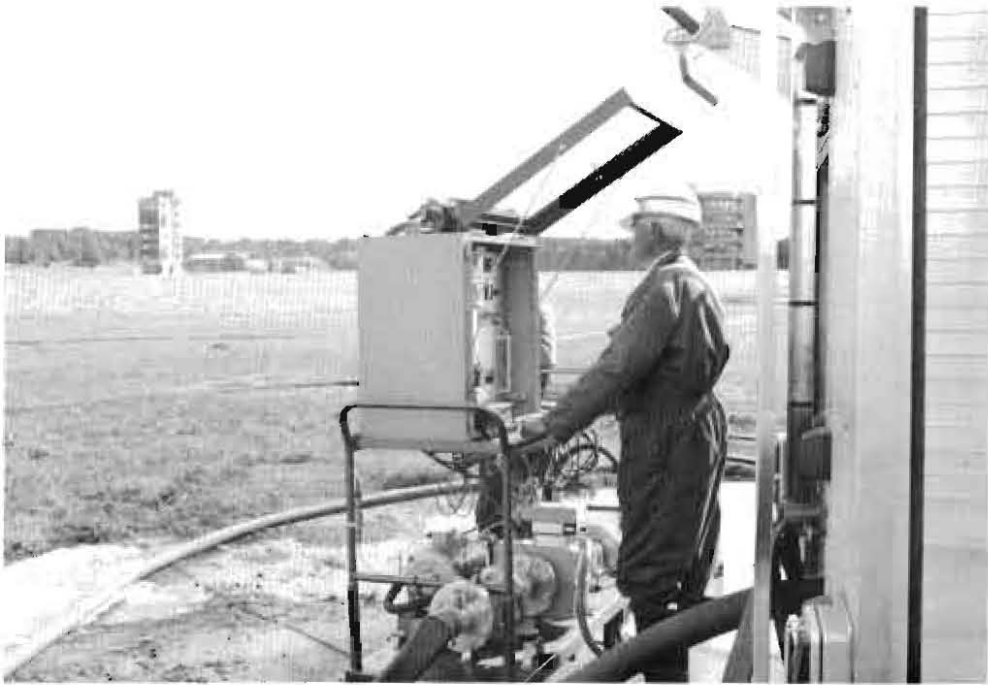
Figure 5: Flowmeter and indicators mounted on trolley
