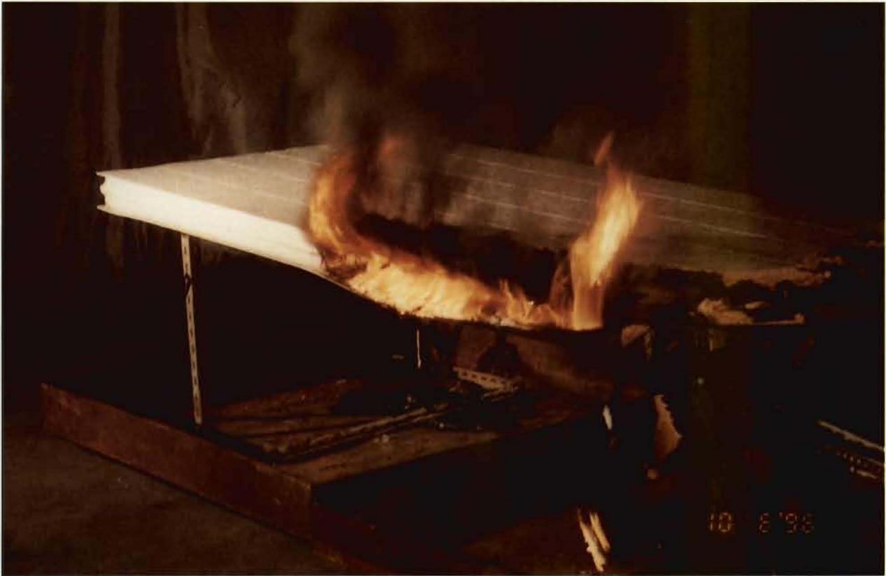
Photo 5. Horizontal Polystyrene Panel Test
