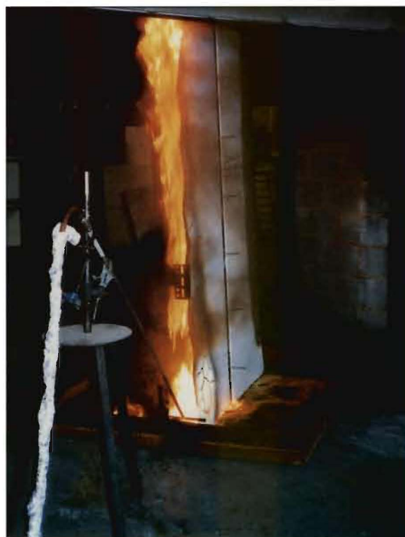
Photo 1. Polystyrene Jointed Panel Test
