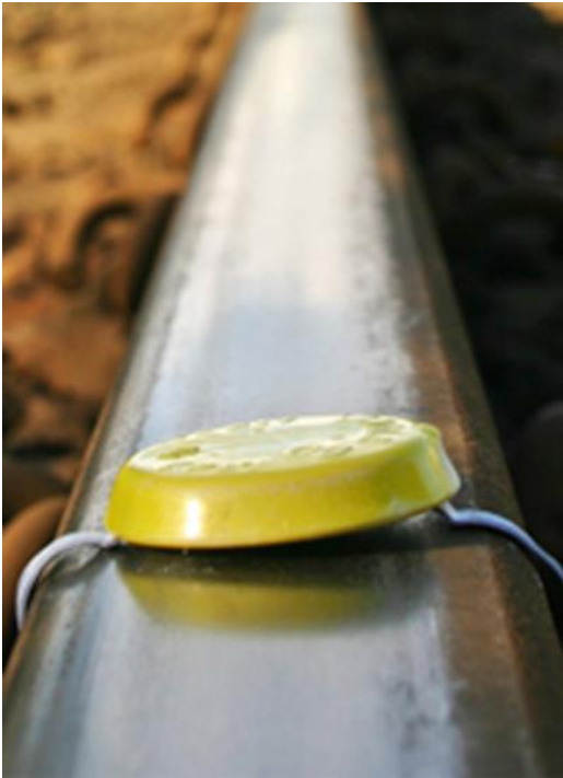
Figure 12: Example of detonator on a rail Source: Open source
